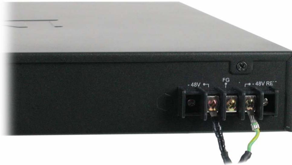
Figure 2 - 5. Power connections attached to contacts after assembly
